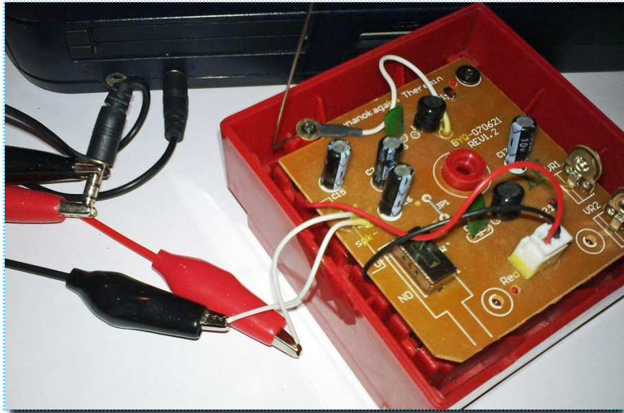
Figure 4.8: The first tested theremin bought from eBay as the cheapest offered there worked out well. The figure shows how the output signal and the audio cable are connected with crocodile clips. On the theremin side, there is only single channel output, and on the soundcard line-in side, only one channel is used from two (second one remains free and can be used to connect one more theremin). The audio cable in the picture has 3.5mm stereo jack plugs at his both sides. The image displays also the simplicity of the theremin hardware
