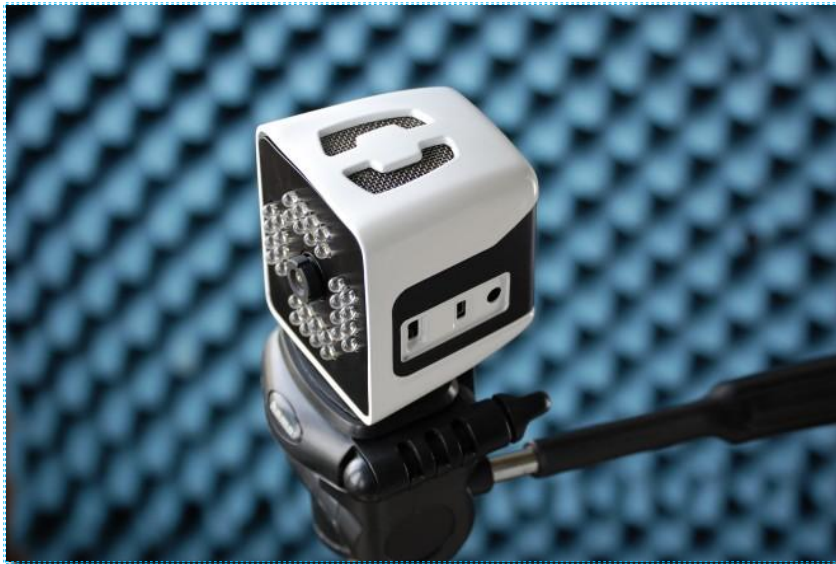
Figure 3.4: Commercial product of infrared time-of-flight depth aware camera produced by Softkinetic
