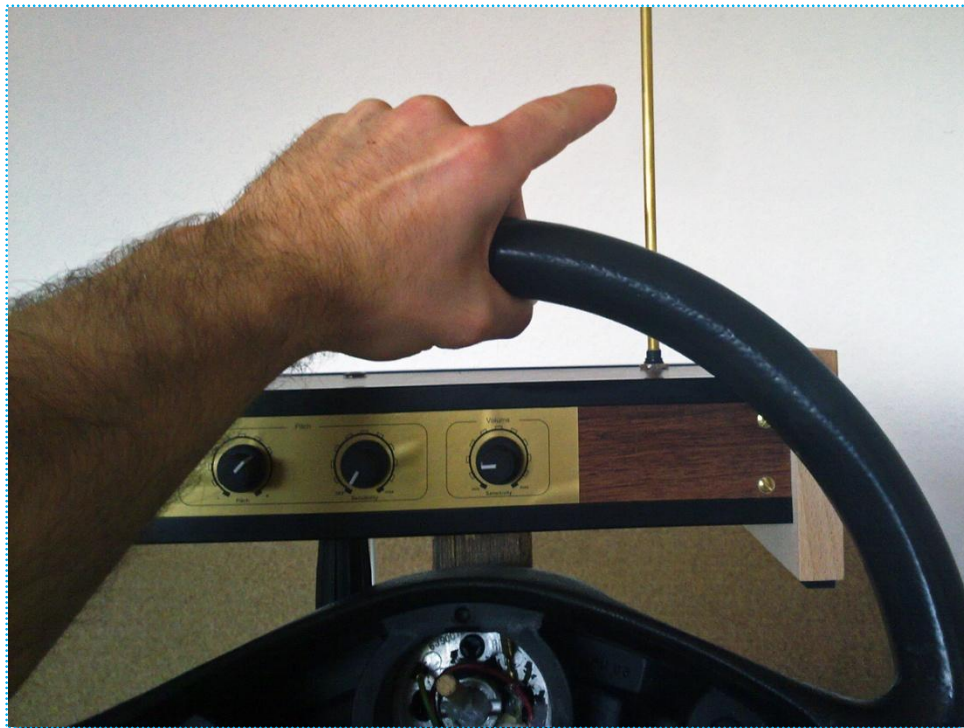
Figure 4.11: The experimental phase represents a typical car situation of holding the steering wheel with left hand and making finger movements, which are to be recognized by the system
